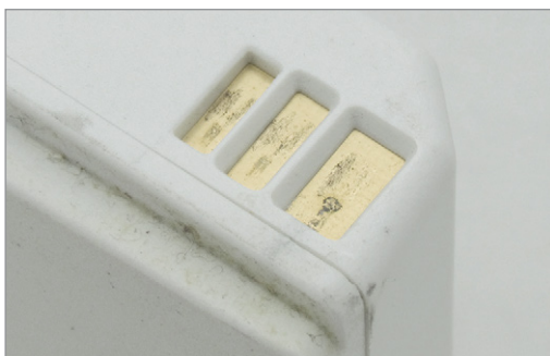
Figure 7. Dirty Battery Contacts
