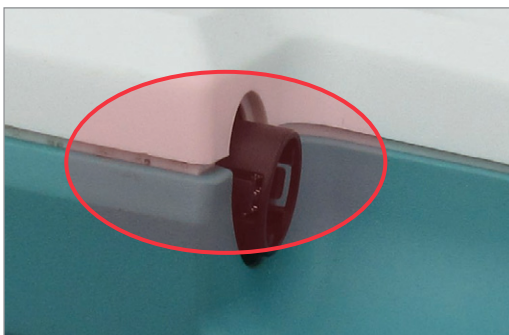
Figure 12. Unacceptable Gap in Assembly
