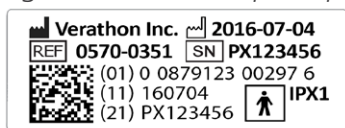
Figure 17. UDI-compliant probe label
