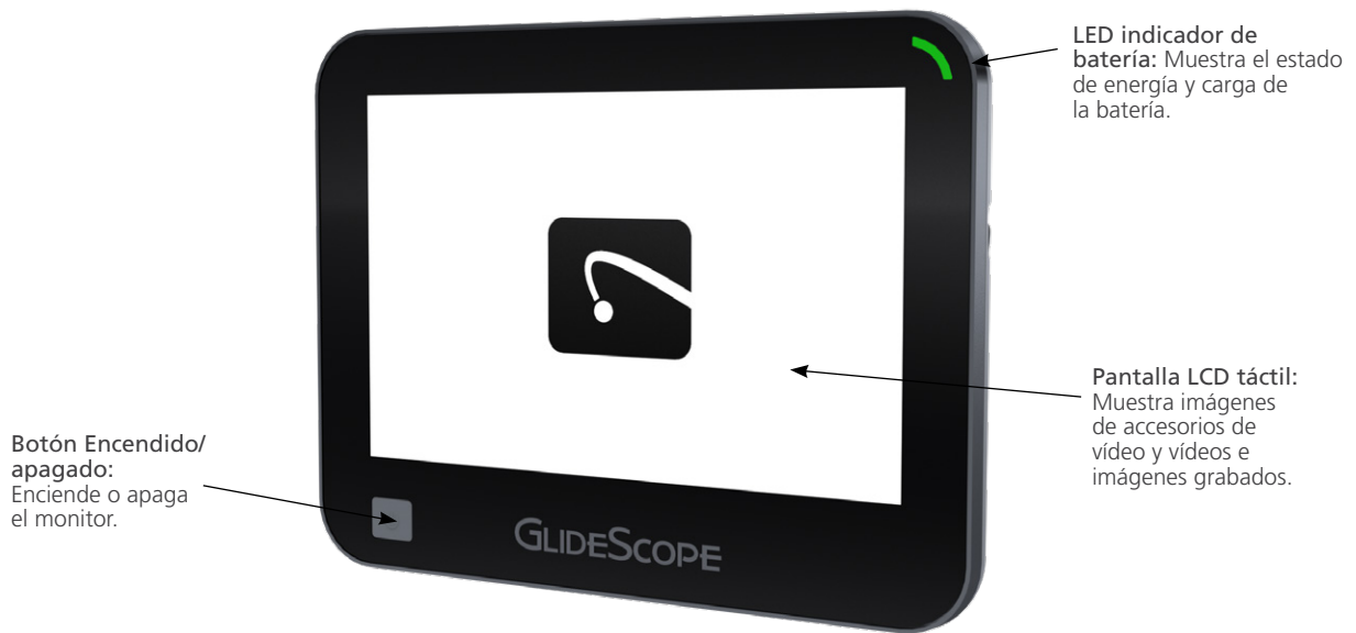
Figura 1. Panel frontal del monitor GlideScope Core
