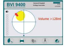
If the scan is unsuccessful, the probe shows an arrow (solid or flashing) indicating the direction to move the probe to be on target.
